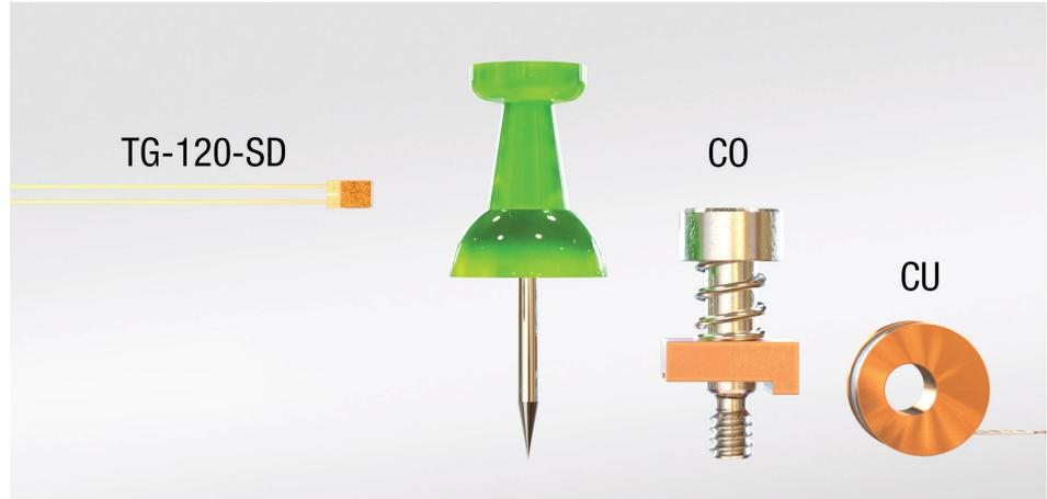
The TG-120 gallium-aluminum-arsenide (GaAIAs) diode temperature sensors are particularly well suited for low to moderate magnetic field applications at low temperatures. The GaAIAs sensing element exhibits high sensitivity (dV/dT) at low temperatures. Voltage-temperature characteristics are monotonic over the sensor's useful range from 1.4 K to 500 K (see data plots below).
